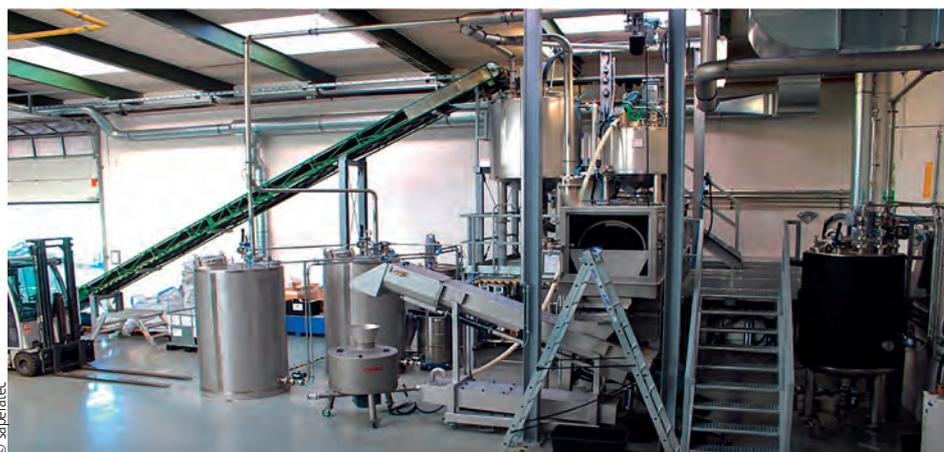
saperatec has developed a process for the delamination of polymer and metal films in flexible packaging materials
