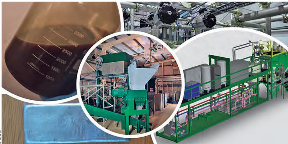
Enval's proprietary process is based on a technology known as Microwave Induced Pyrolysis
